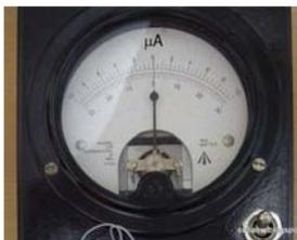
I repeated the circuit to demonstrate that I can use my DVOM as a centre-zero meter. I just have to rotate the potentiometer slowly .
