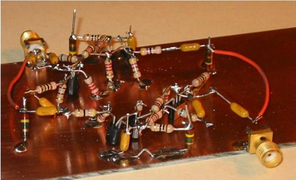
**Fig 4. Photo of the amplifier from Fig 3. SMA connectors were used to facilitate measurements while ugly construction allowed a quick build.**
